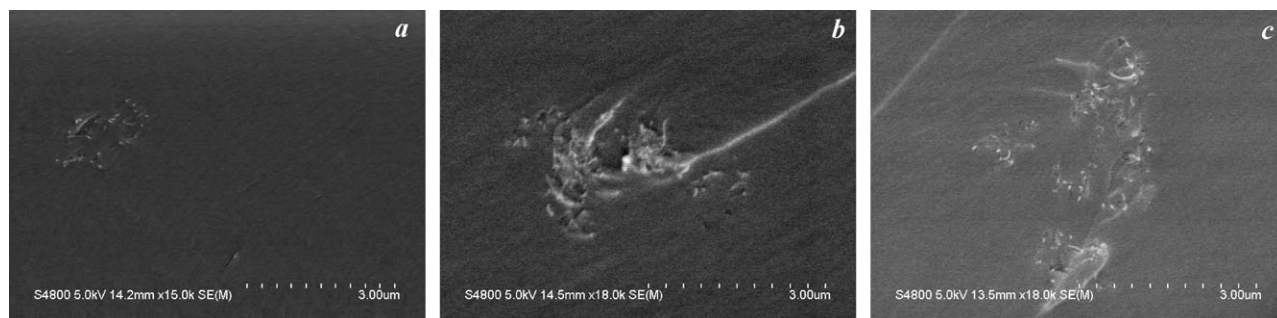
Figure 2. SEM micrograph of epoxy NC with 1 (a), 1.9 (b), and 3.8 (c) wt % of MWCNTs.
